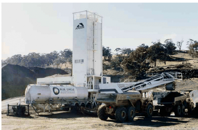
Above: The Aran MODUMIX II-4 mixing plant producing RCC. The same machine can mix structural and slipform concrete with equal efficiency.
